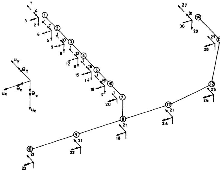
FIG. 3. Finite element model for the antisymmetric motion.
