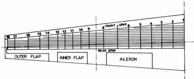
FIG. 4. Wing structural details of the aircraft.
