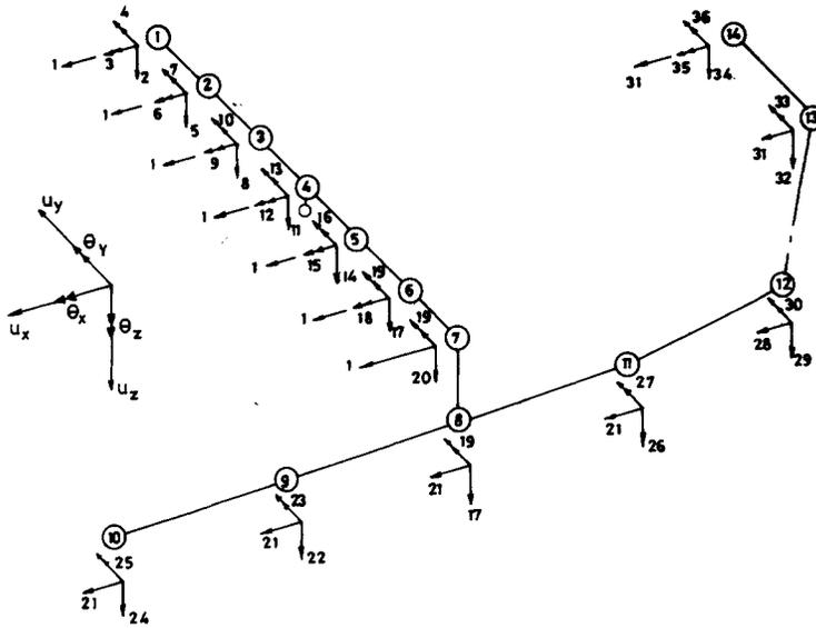
FIG. 2. Finite element model for the symmetric motion.
