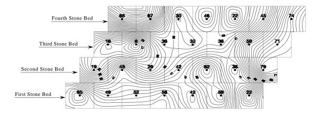
Figure 5. A representative contour map showing low & very low deterioration category in the four studied stone beds of Khufu Pyramid
