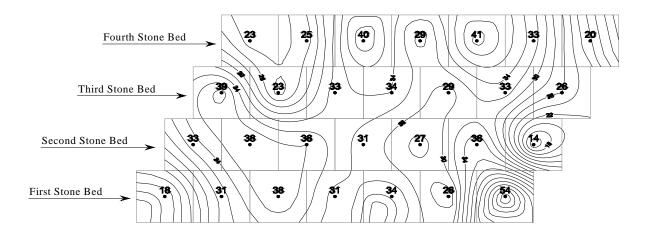
Figure 4. A representative contour map showing medium deterioration category in the four studied stone beds of Khufu Pyramid
