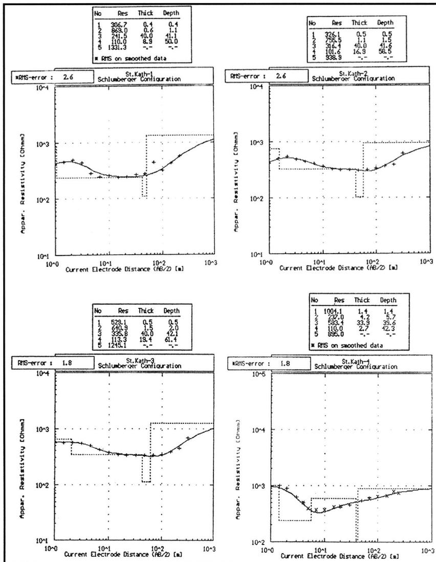
Fig. 10 a. Resistivity sounding field data and the calculated resistivity models of soundings (1, 2, 3 and 4).
