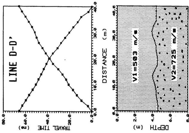
Fig. 6. Travel-time and corresponding velocity depth section of seismic refraction line D-D'.
