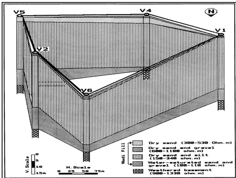
Fig. 11. Resistivity panel diagram for the interpreted resistivity models.
