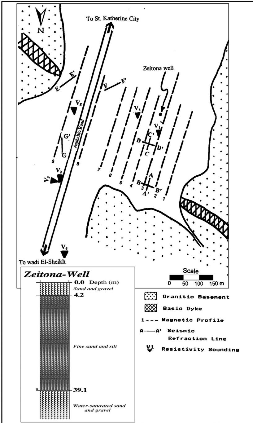
Fig. 2. Layout of the applied geophysical tools.
