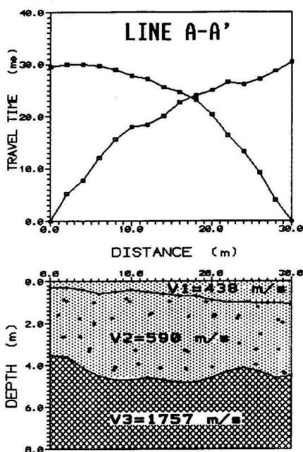
Fig. 3. Travel-time and corresponding velocity depth section of seismic refraction line A-A'.
