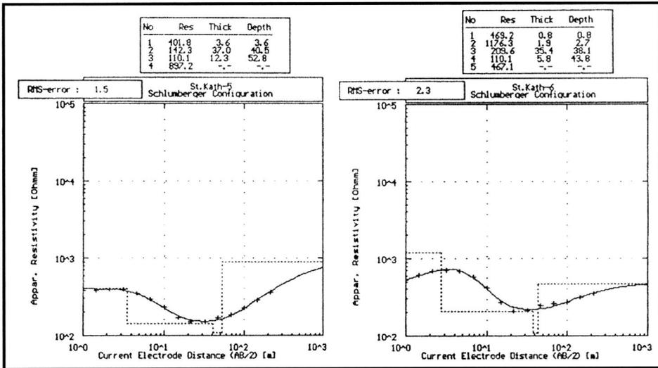
Fig. 10 b. Resistivity sounding field data and the calculated resistivity models of soundings (5 and 6).
