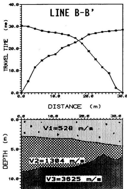
Fig. 4. Travel-time and corresponding velocity depth section of seismic refraction line B-B'.
