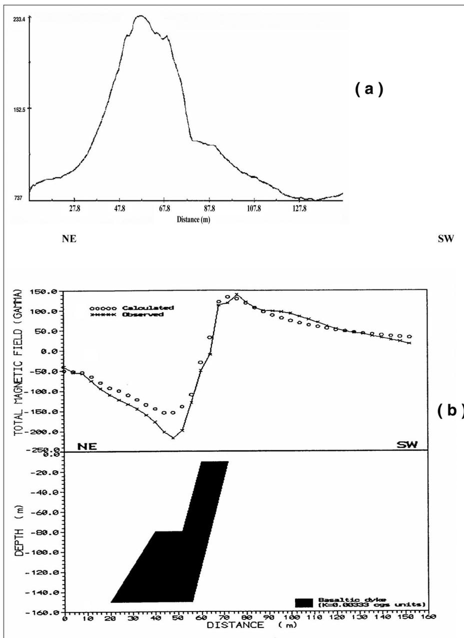
Fig. 13. Analytical signal analysis (a) and 2½-D magnetic model (b) for the magnetic profile shown in Fig. (12a).
