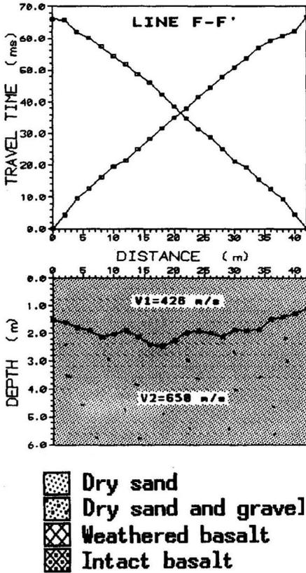
Fig. 8. Travel-time and corresponding velocity depth section of seismic refraction line F-F'.
