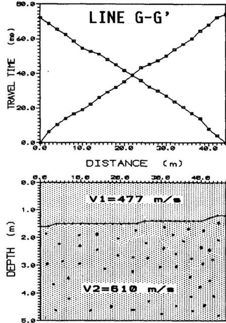
Fig. 9. Travel-time and corresponding velocity depth section of seismic refraction line G-G'.
